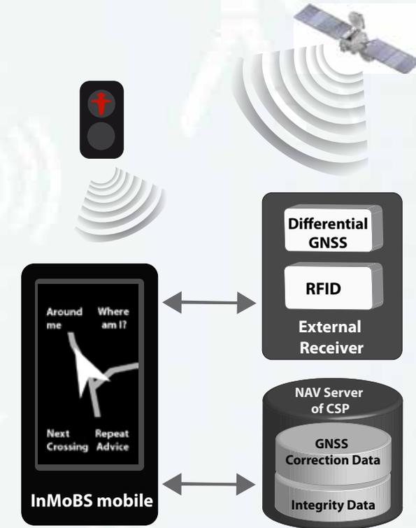
Using an external GNSS receiver a more accurate positioning within 1 to 3 m is possible. Therefore the receiver uses differential GNSS correction data which are provided by the Component Server Platform. The positioning solution is supported by the RFID technique; i. e. small transmitter integrated in the traffic lights allowing additional reliability on crucial waypoints.
